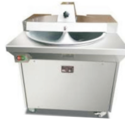
QXP 30 Bowl Chopper Power: 550w Size: 770x710x960mm Cap.: 20 Ltrs.
